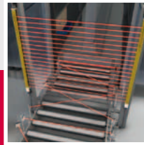
Hand and finger protection — MLC safety light curtain
